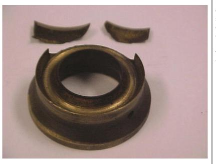
The discoloration of the brass retainer indicates heat which is caused by a restriction of water supply to pump. This restriction causes cavitation, which damages the inside of the pressure packing, and transfers this implosion force outward to the brass retainer.
